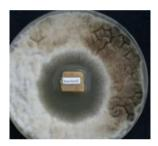
The photo on the left shows a sample of Sterishield modified Sureshield in a agar media fully inoculated with mould (Aspergillus) this is growth after three days.
